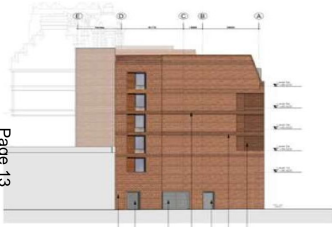
01 - East Elevation Gable Wall
